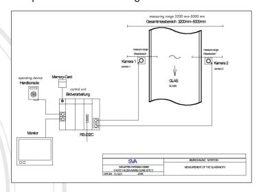
The SVA system enables you to measure the width of the glass in a range between 3200mm and 5200mm.
